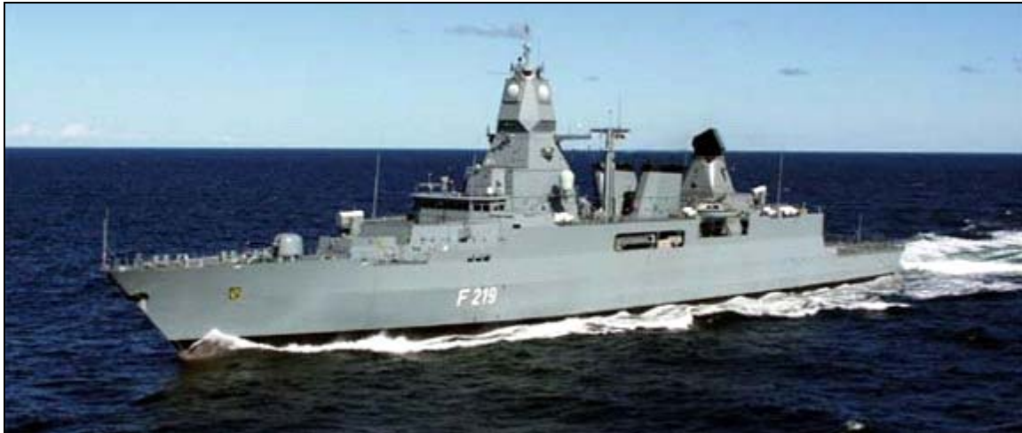
Germany's F-124 Class Frigate Sachsen Mounted with the APAR Multifunction Radar
