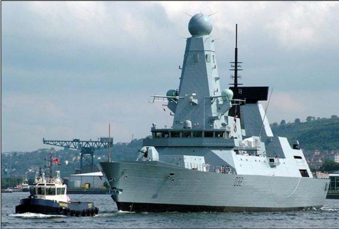
The Type 45 Destroyer HMS Daring Equipped with Sampson Radar during Sea Trials
