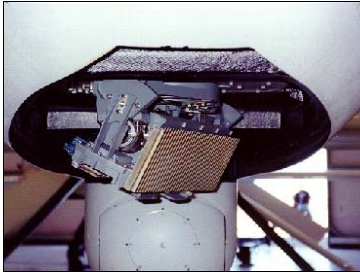
The ZPQ-1(V) TESAR Radar
