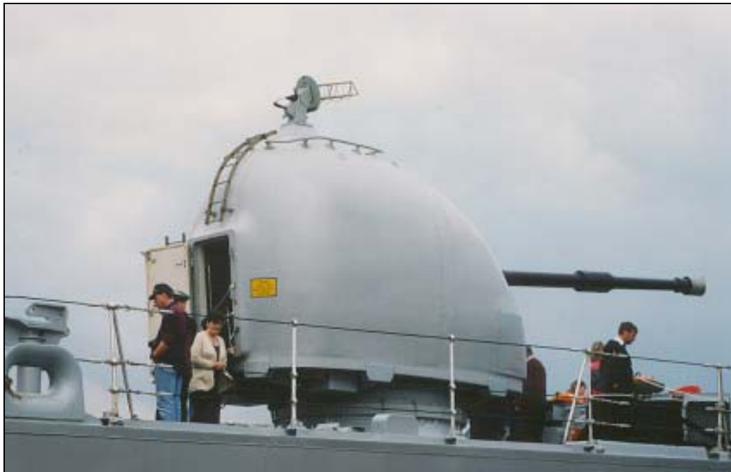
4.5-Inch L55 Mk 8 Gun. (Note antenna for experimental course-corrected shell program.)
