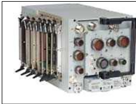
Link 16 MIDS Tactical Data Link Terminal Made by ViaSat
