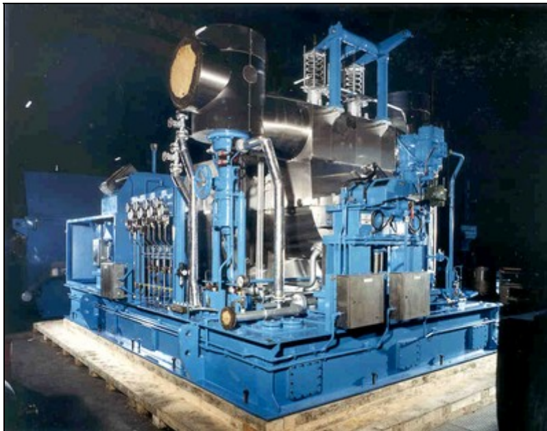
20-MW backpressure turbine installed in a sugar mill in Zimbabwe.
