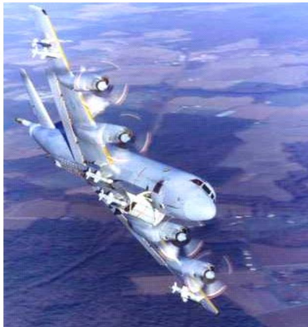
Lockheed-Martin P-3C Orion maritime patrol aircraft of US Navy is one of the primary platforms carrying the ASQ-81/ASQ-208 MAD system
