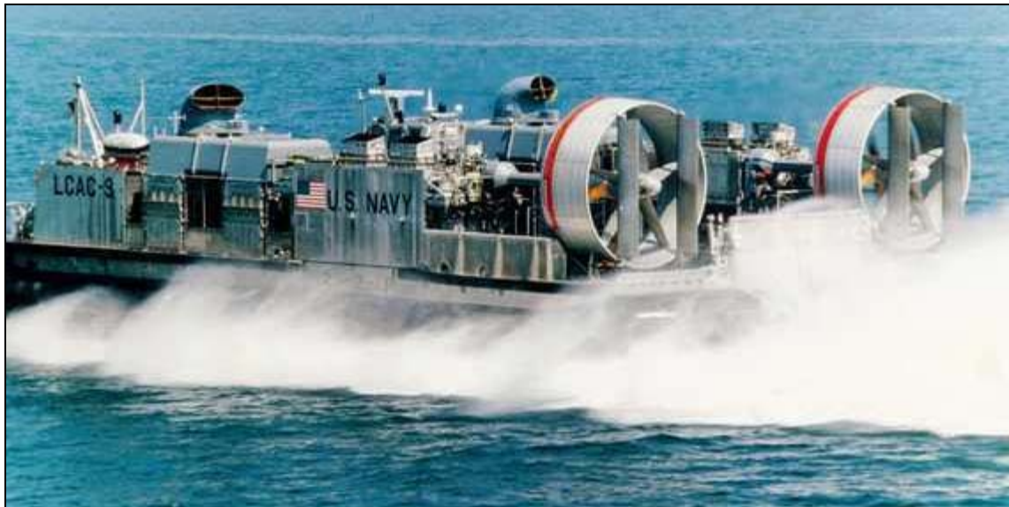
The LCAC is powered by four TF40B gas turbines.
