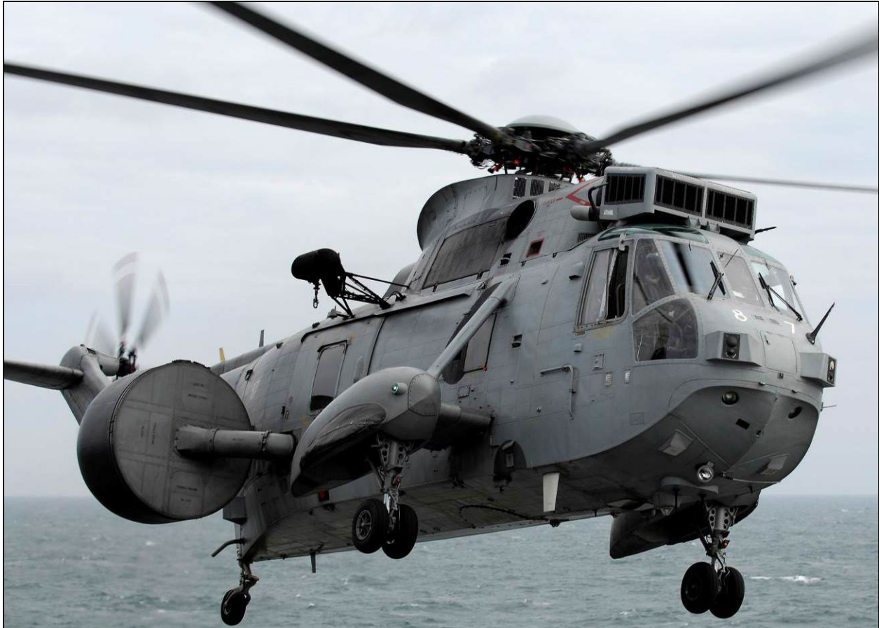
U.K. Royal Navy Sea King AEW Helicopter, Featuring the Telltale Searchwater Radome in a Retracted Position Aft of the Cabin Door
