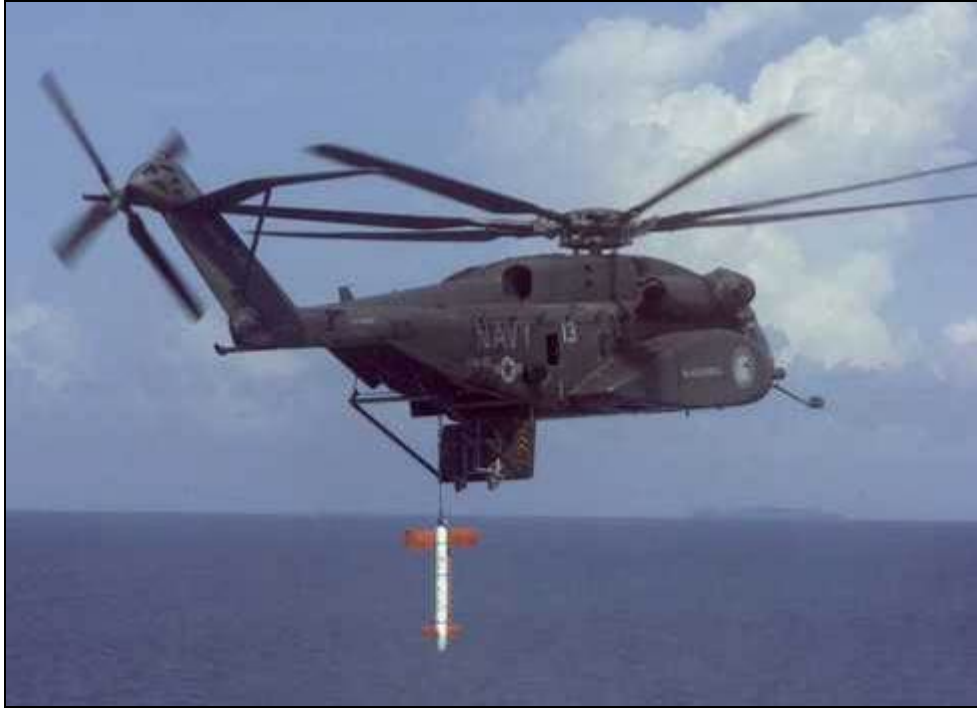
AQS-14A Minehunting Sonar System Being Deployed from a U.S. Navy MH-53E Sea Dragon Helicopter
