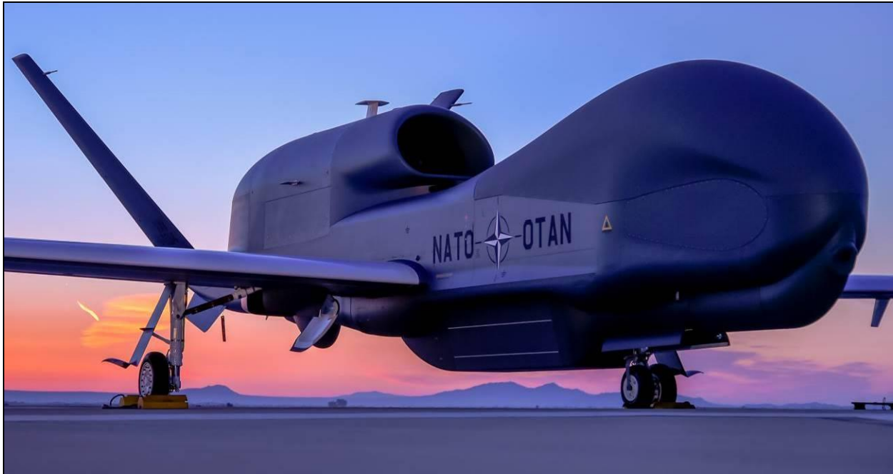
The Global Hawk Block 40-based NATO AGS UAV features the ZPY-2 MP-RTIP.
