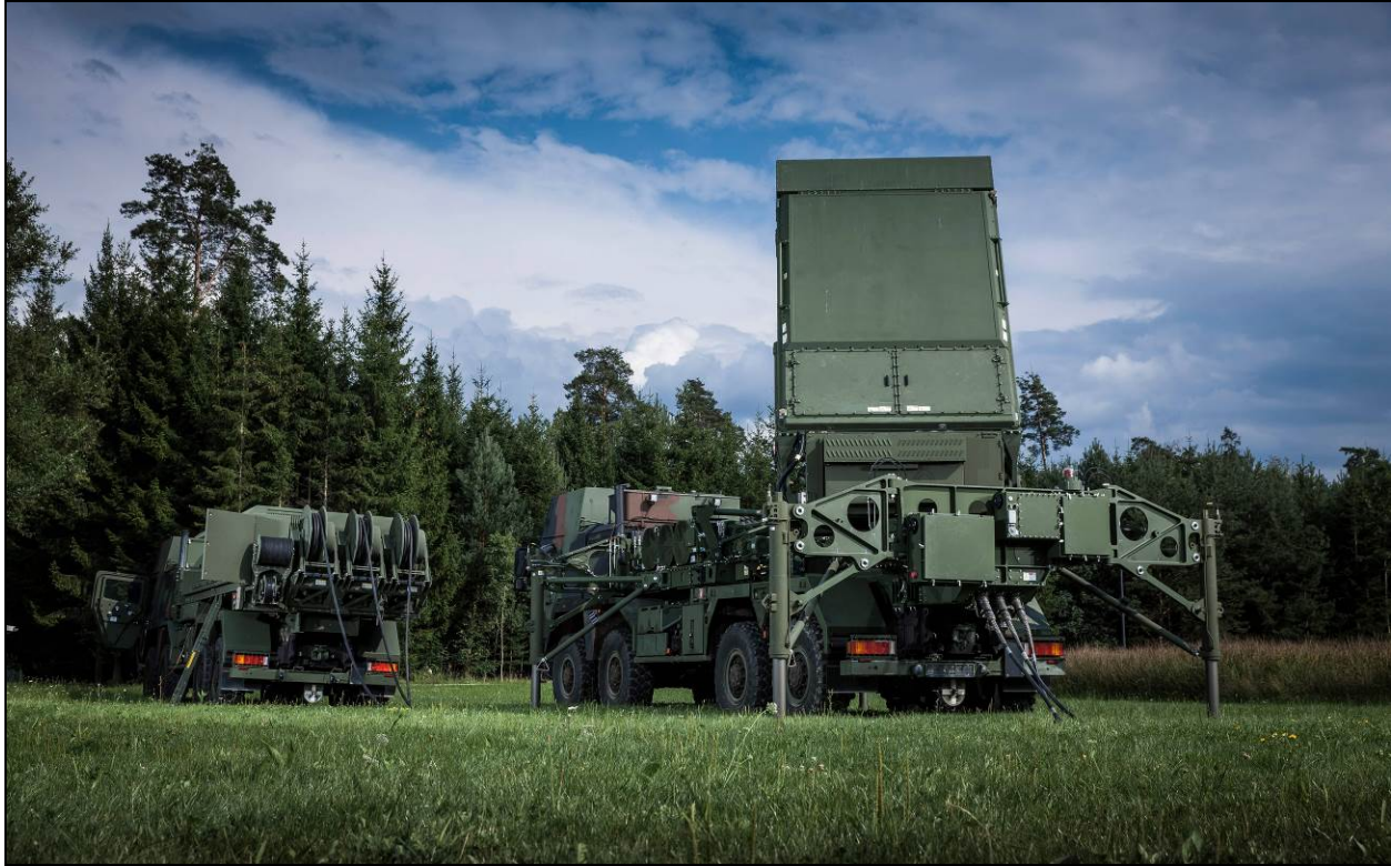
The MEADS Fire Control Radar and Auxiliary Power Unit
