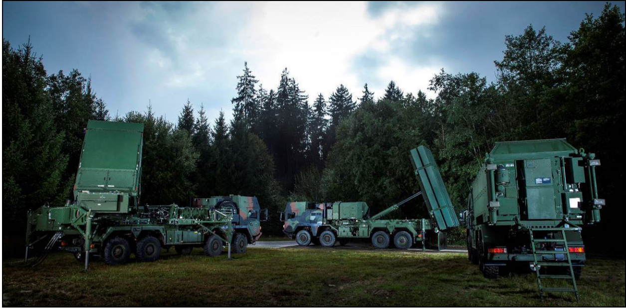
The Complete MEADS Air Defense System, with the Radar Truck to the Left
