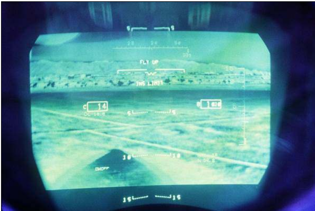
Infrared Imagery from LANTIRN Projected on the HUD of a USAF F-15E
