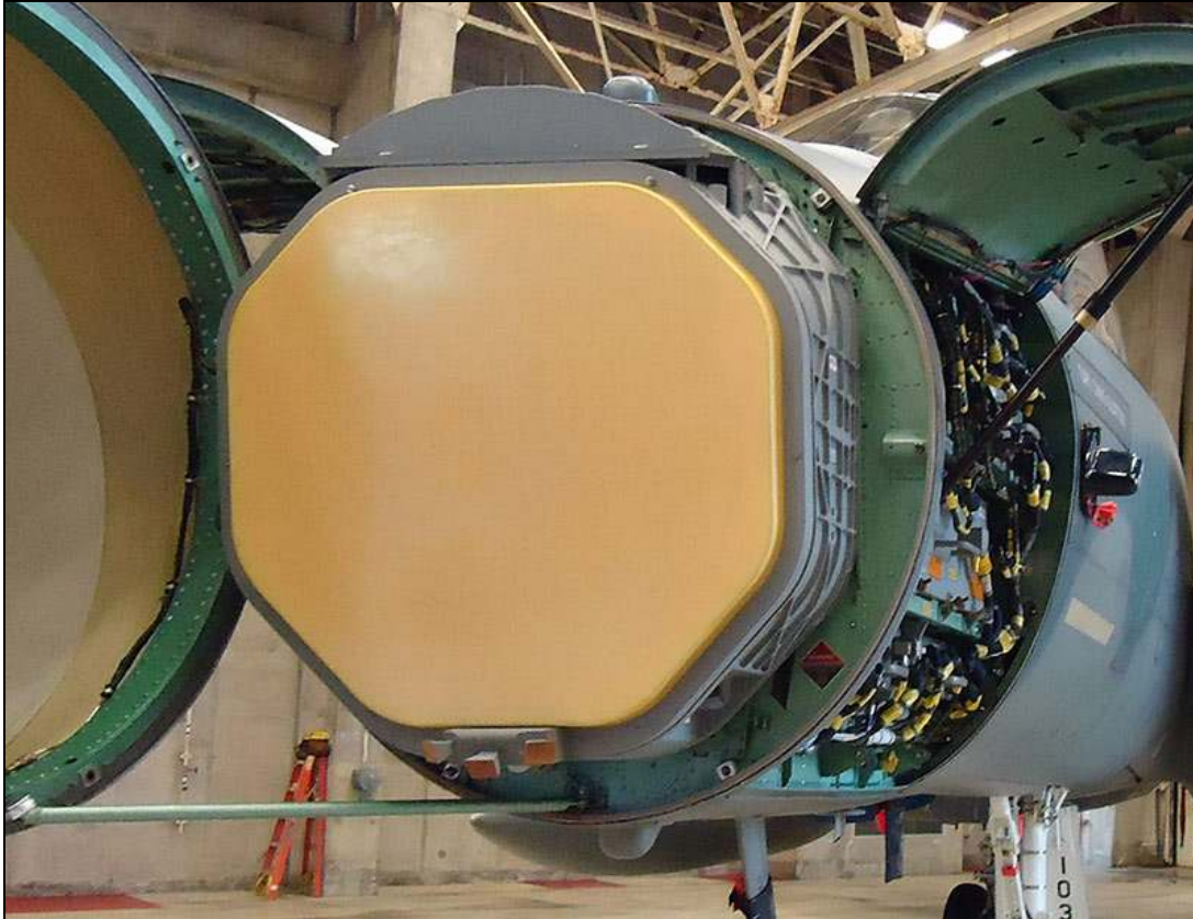
APG-63(V)3 in an F-15C Nosecone
