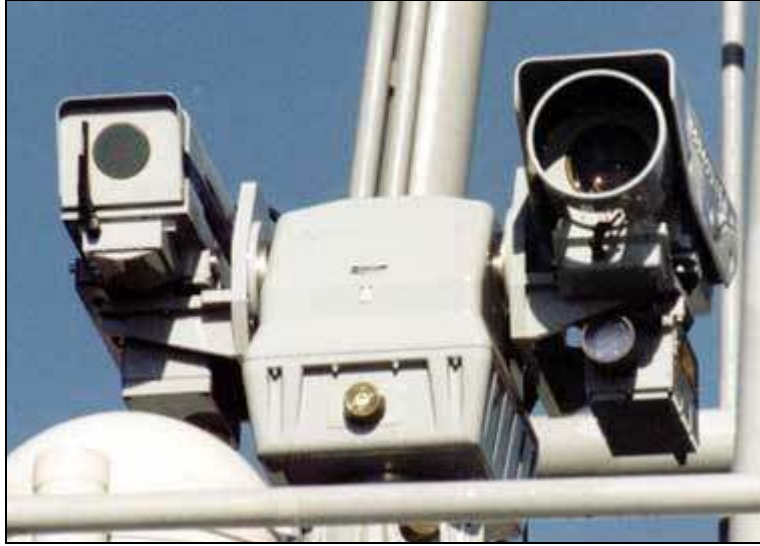
Radamec System 1500 Naval Electro-Optical Tracking and Fire Control System
