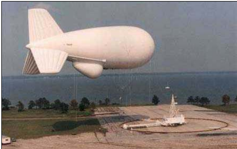
The JLENS consists of an aerostat equipped with advanced radar systems.
