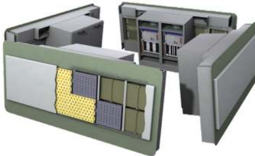
The Active Phased Arrays of the IM400's SMILE/Sea Master 400 Long-Range Surveillance Radar
