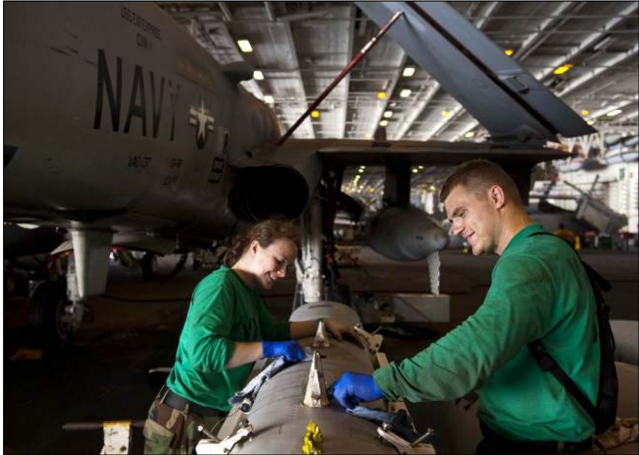
Two U.S. Navy technicians service an ALQ-99 pod.
