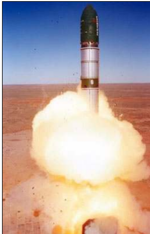
A Converted SS-18 Dnepr Launch Vehicle
