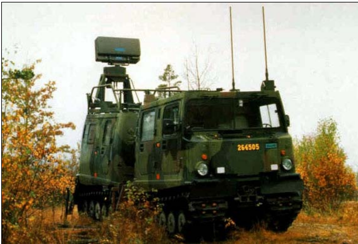
Saab Microwave Systems' HARD Radar Mounted on a Hägglunds BV-208 All-Terrain Vehicle
