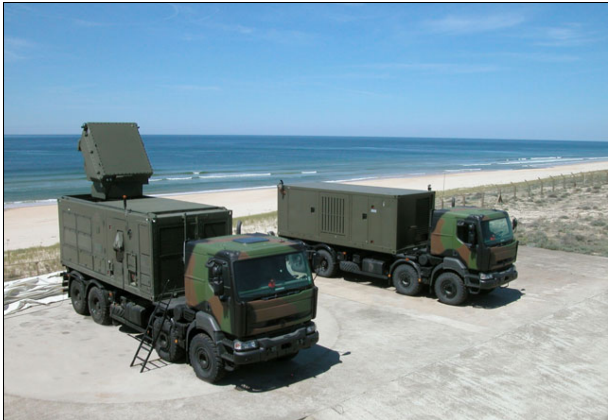
Arabel Radar as Seen as Part of the SAMP/T System
