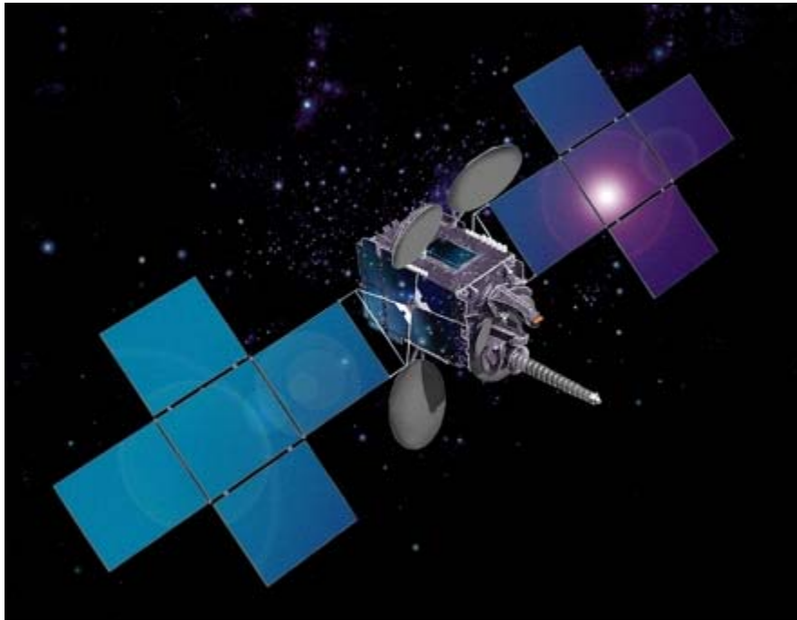
Satmex 6 was built by Space Systems/Loral on the company's FS1300 bus.
