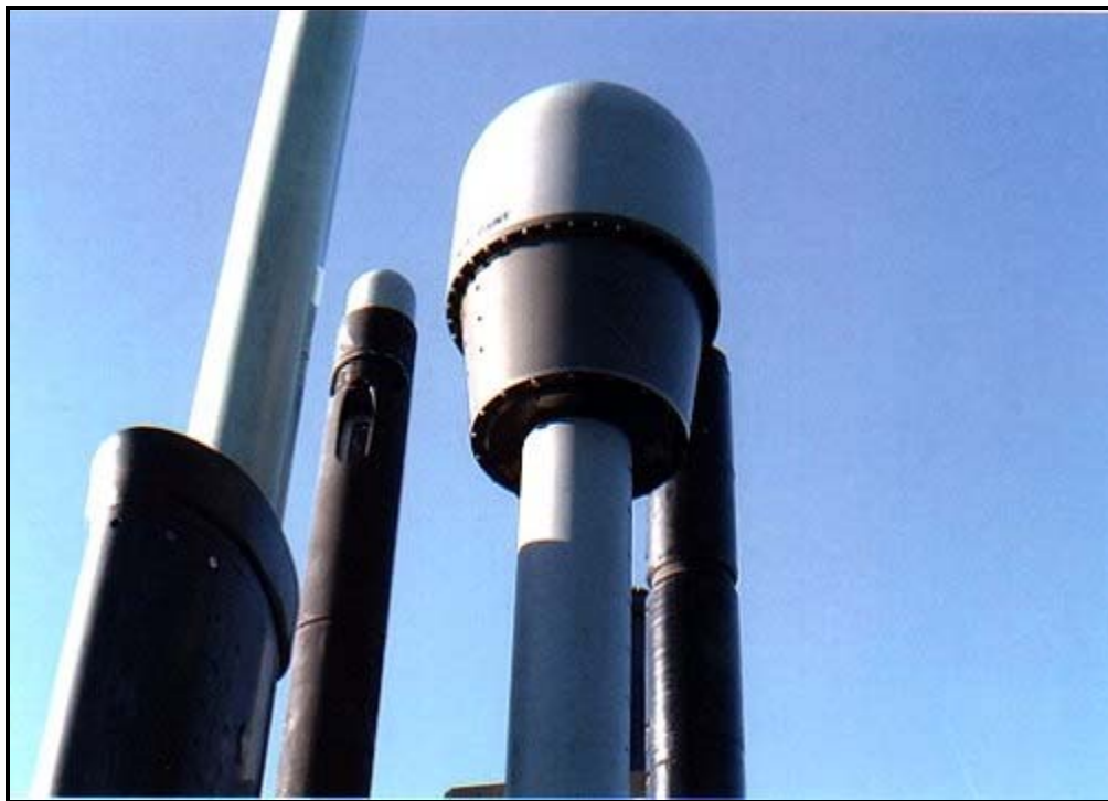
Extremely Low Frequency (ELF) submarine communications. The SubHDR Antenna Installation on USS PROVIDENCE (SSN 719). The current periscope mounted system is just to the left of the larger SubHDR antenna
