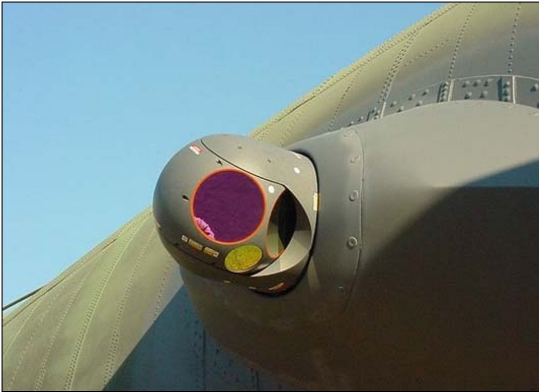
DIRCM System Installed on MC-130
