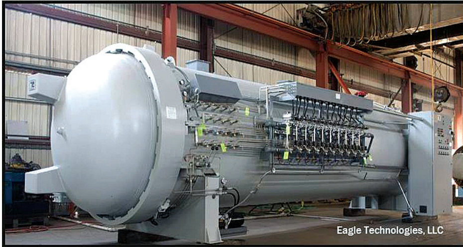
Eagle Technologies has an in-house autoclave capability with a 5 ft (1.5 m) diameter and a 27 ft (8.2 m) inside length. (Eagle photo)
