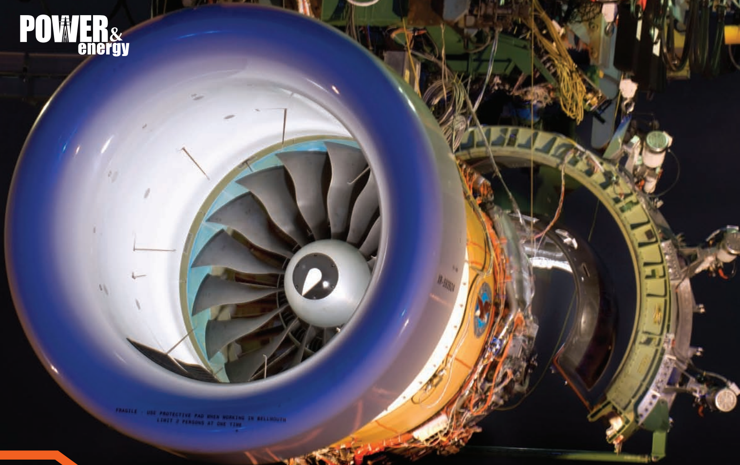
The Pratt & Whitney geared turbofan engine, shown being readied for a test, may reduce aircraft noise at takeoff by 77 percent.
