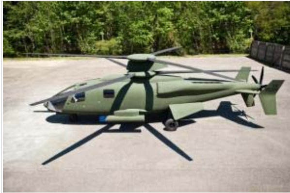
A mockup of Sikorsky's X2 Technology Light Tactical Helicopter offers technology that enables aircraft to fly at higher speeds with counter-rotating main rotors on top and an auxiliary propeller at the back. (contributed photo)
