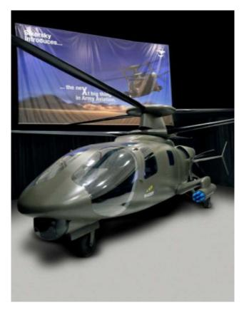
A mock up of what Sikorsky Aircraft expects its S-97 Raider to look like. It is the new hybrid helicopter, the company is building after successful tests of an experimental aircraft that uses similar technology, the X2. Photo: Steven Kaeter ©Pratt & Whitney, Steven Kaeter / Connecticut Post Contributed
