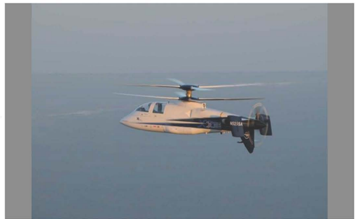
The Sikorsky's X2 has two counter rotating blades on top of the aircraft and a prop that pushes from behind This was the 17th flight of the X2, an aircraft wholly funded by Sikorsky. Photo: Contributed Photo/C. David LaBianca , Contributed Photo/C. David LaBianca / Connecticut Post Contributed C. David LaBianca
