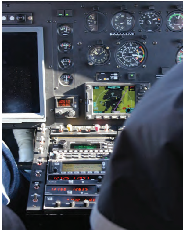
To date, Honeywell has delivered more than 2,000 helicopter EGPWS units. The display provides the pilots with real time maps of terrain.
