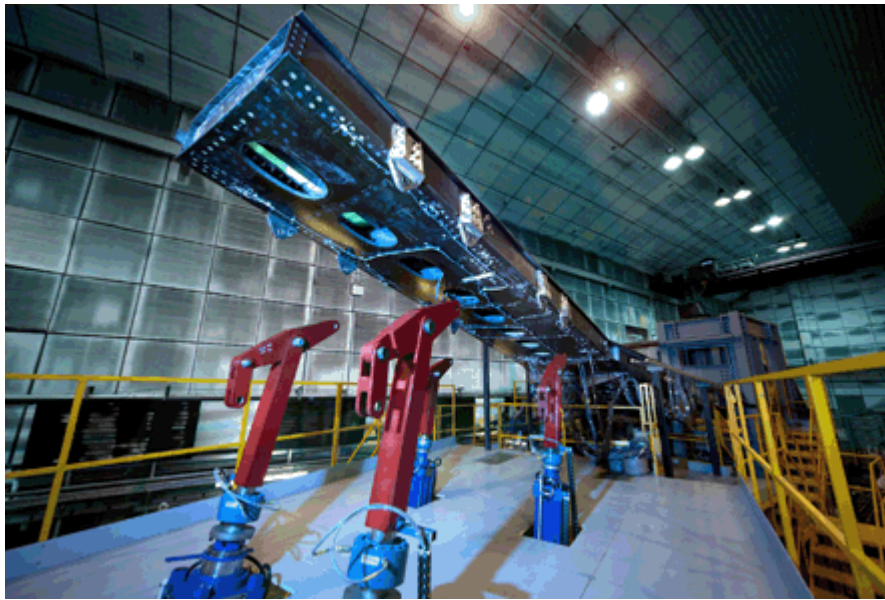
The carbonfibre wing demonstrator is tested to its limit in Belfast
