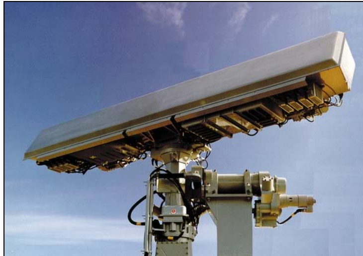
Type 996/AWS-9 E/F-band surveillance and targeting radar
