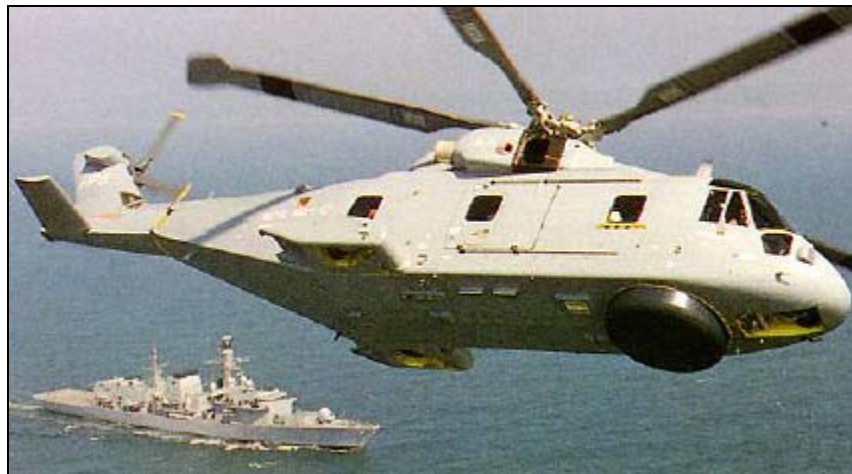
Blue Kestrel radar dome visible on underside of helicopter
